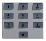
Using the numeric keys, you can enter a user name, similar to typing a text message on a mobile phone. Use '0' key for space.
