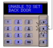
An appropriate **A B C D** key will flash to indicate within which area the fault exists.
