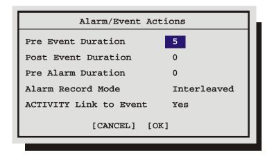
**Pre Event Duration:** The unit will record up to 5 seconds of data ahead of the event trigger, at the Event Record Rate. Select from 0 to 5 seconds.
